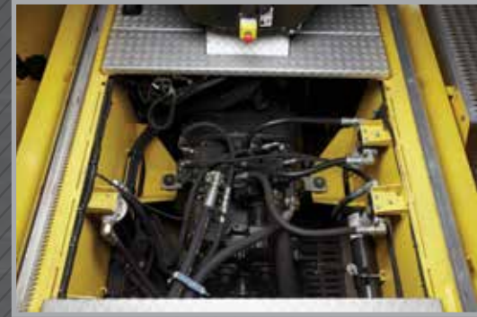
Load-sensing on-demand hydraulic system
