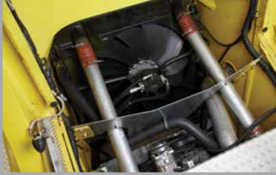
Cooling system with puller fan
